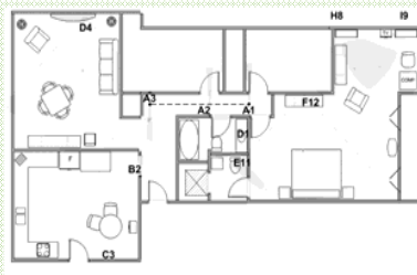
Strategically placed arrays of passive infra-red motion sensors, contact door sensors, and home PC.
